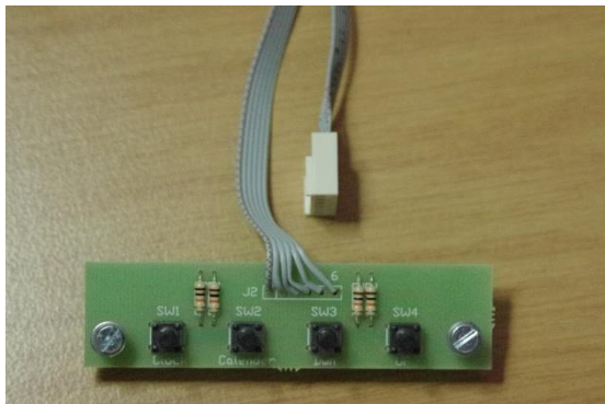
This is the switch Pc Board to allow you to set the time and Date.
